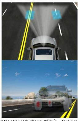
continuous and dashed – in daylight and at night and operates at speeds above 70km/h. At lower speeds, typical of urban driving, the system is disabled in order not to irritate or distract the driver with unnecessary warnings.
