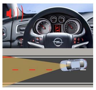
are sufficiently distinct, unmarked road edges. The warning signal and a blinking icon on the instrument panel are suppressed if the system detects that the driver is intentionally leaving the lane: the driver's use of the direction indicators, steering, brakes and accelerator are used to determine whether the lane departure is deliberate or not. If Opel Eye is not able to detect a lane, the driver is warned that the system is not able to assist.
