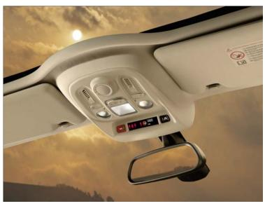
then establishes a voice connection between the car and the call centre, allowing the vehicle's occupants to communicate with a trained operator. If the occupants of the car are unconscious or otherwise unable to communicate, the call centre immediately notifies the emergency services and provides information about the location of the accident. Otherwise, the operator establishes the extent of the occupants' injuries and decides whether or not the emergency services should be notified.
