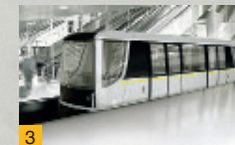
3 Great speed: The automated people mover (APM) connects the satellite with Terminal 2 via two 400-meter-long underground tunnels with a journey time of just one minute.
