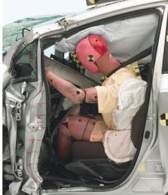
The Suzuki Kizashi (far left) earns a good overall rating and is the only midsize moderately priced car with a good rating for structure. There was only minor intrusion into the occupant compartment. In contrast, survival space for the driver in the Toyota Prius v (left) was seriously compromised. The side curtain airbag also deployed too late to offer protection. The Prius v earns a poor rating.
