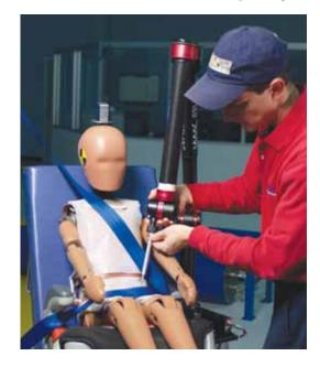
An engineer at the Institute's Vehicle Research Center evaluates how lap and shoulder belts fit a test dummy representing an average-size 6-year-old child under four conditions representing a range of belt configurations in real-world vehicles.
