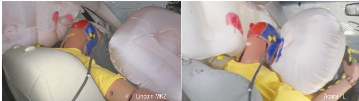
The dummy's head and chest missed the MKZ's front airbag as the steering column moved to the right. The side curtain airbag didn't have sufficient forward coverage for the head.
