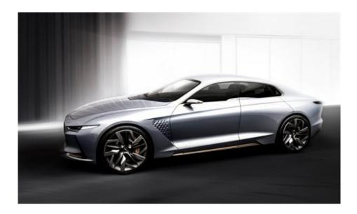
Acknowledging the Genesis brand's sporty and agile nature, the hybrid concept generates 245ps and 36.0 kgf.m of torque from its 2.0 T-GDi powertrain coupled with an 8-speed automatic transmission. The advanced technological features and precise design language of the concept emphasize key aspects of Korean culture, while elevating the value and perception of the Genesis brand.
