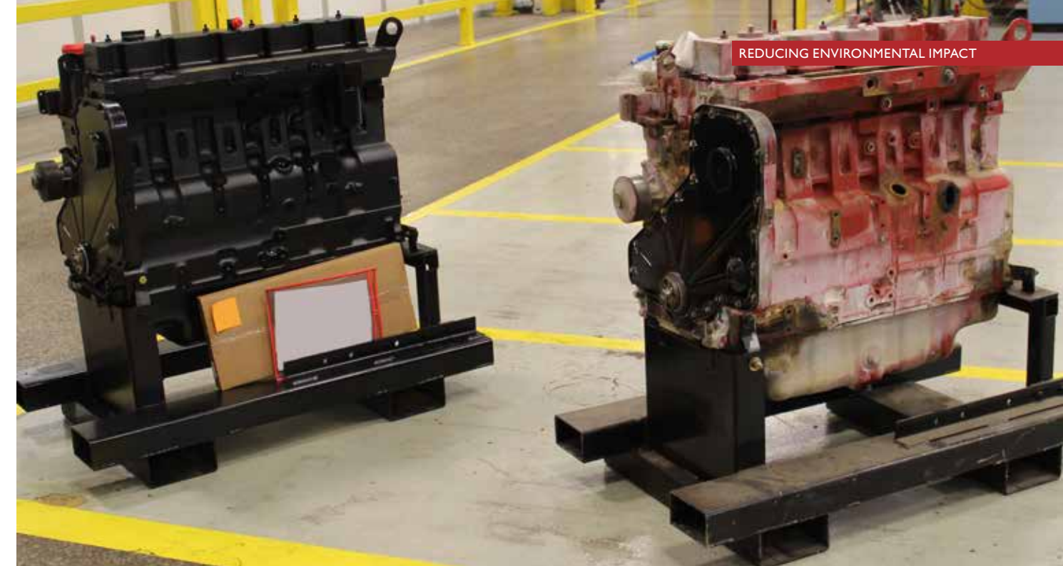
An engine before remanufacturing (right) and once the remanufacturing process has been completed (left)
