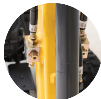
The E17C, E26C, E33C and E37C feature a standard hammer circuit and selectable 2-way auxiliary hydraulics.
