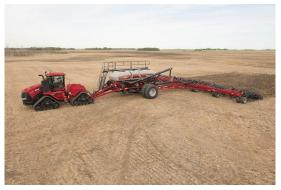
Photo caption: The new Case IH Precision Air<sup>™</sup> 4585 air cart features a four-tank design with a total capacity of 580 bushels.
