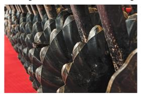
Caption: The Case IH True-Tandem<sup>™</sup> 335 Barracuda vertical tillage system moves material up, over and laterally to stratify soil particles and increase aeration for improved soil tilth.
