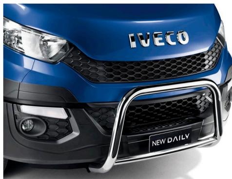
The New Daily also features a **complete protection system**: it contains a “pushbar” and side protection bars to increase both active and passive safety of the vehicle and pedestrians in case of incident.
